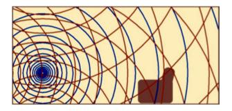
By contrast, the **Wisdom Sage Series L75m** speakers radiate sound as a "line source". The sound moves into the room as an expanding cylinder, rather than as an expanding sphere – as though from a vertical line suspended in space.
