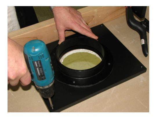
4) Align the \$55/\$90 flange plate on the \$55/\$90, flush with the corner of the enclosure, and screw into place.
