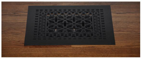
One important characteristic of any replacement HVAC grille or grate you may elect to use for aesthetic reasons: many such grille have adjustable louvres to direct the flow of air. These should be either removed or frozen in place with liberal amounts of glue in order to avoid rattles. A lot of air will be flowing through these grilles, in both directions. Anything that can rattle, will rattle.
