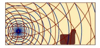
By contrast, the **Wisdom Series L75m** speakers radiate sound as a "line source". The sound moves into the room as an expanding cylinder, rather than as an expanding sphere – as though from a vertical line suspended in space.
