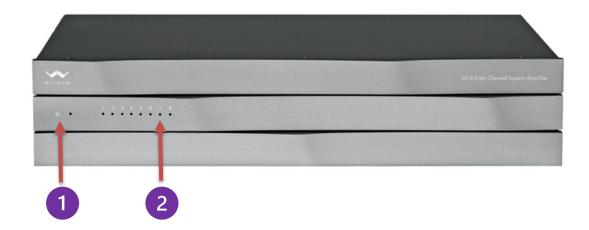
1. Power Switch and Indicator: The SA-8 features a sculpted front panel that conceals a switch under the flexible left end of the middle section. Gently pressing the left end of the center section will engage a micro switch under the face of the SA-8, which will in turn toggle the unit between operate and standby. The international symbol for power is inscribed in this location to designate its purpose.
