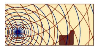
By contrast, the **Wisdom Series LS4m** speakers radiate sound as a "line source". The sound moves into the room as an expanding cylinder, rather than as an expanding sphere – as though from a vertical line suspended in space.
