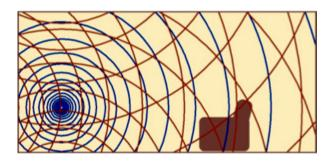
By contrast, the **Wisdom Series L150i** speakers radiate sound as a "line source". The sound moves into the room as an expanding cylinder, rather than as an expanding sphere – as though from a vertical line suspended in space.
