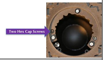
3: Install the Spiral Planar Magnetic Driver (ICS-SPMD). The ICS3-SPMD can only be inserted in one way to make the electrical connection.
