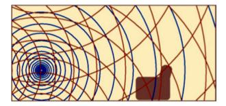
By contrast, the **Wisdom Series L75i** speakers radiate sound as a "line source". The sound moves into the room as an expanding cylinder, rather than as an expanding sphere – as though from a vertical line suspended in space.
