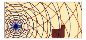
By contrast, the **Wisdom Series L75** speakers radiate sound as a "line source". The sound moves into the room as an expanding cylinder, rather than as an expanding sphere — as though from a vertical line suspended in space.
