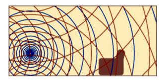
By contrast, the **Wisdom Series L100i** speakers radiate sound as a "line source". The sound moves into the room as an expanding cylinder, rather than as an expanding sphere – as though from a vertical line suspended in space.
