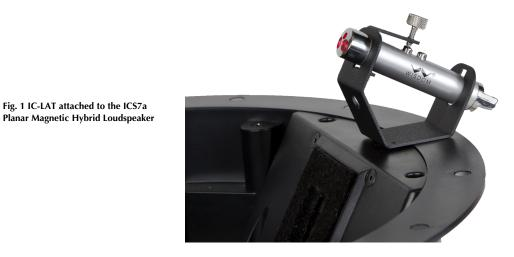
8. If the IC-LAT Laser is used: Turn the laser on the IC-LAT on by rotating the thumbscrew slowly in a counter-clockwise direction until the laser is activated. Rotate the speaker module until the IC-LAT laser is pointing to the desired listening position. Tighten the four screws that control the dog-ears until the speaker module is fixed tightly to the ceiling.
