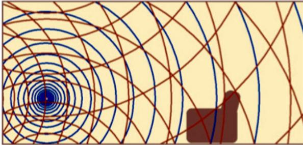
By contrast, the **Sage Cinema Series Line 3** speakers radiate sound as a “line source”. The sound moves into the room as an expanding cylinder, rather than as an expanding sphere — as though from a vertical line suspended in space.
