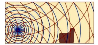
By contrast, the **Wisdom Series LS3m** speakers radiate sound as a "line source". The sound moves into the room as an expanding cylinder, rather than as an expanding sphere — as though from a vertical line suspended in space.
