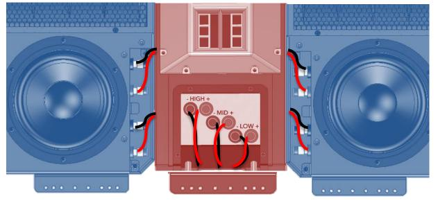
Three pairs of speaker wires from the amplifier are needed. One for Low, one for Mid, and one for High. Route wires through the access panel in the rear of the Center Module
