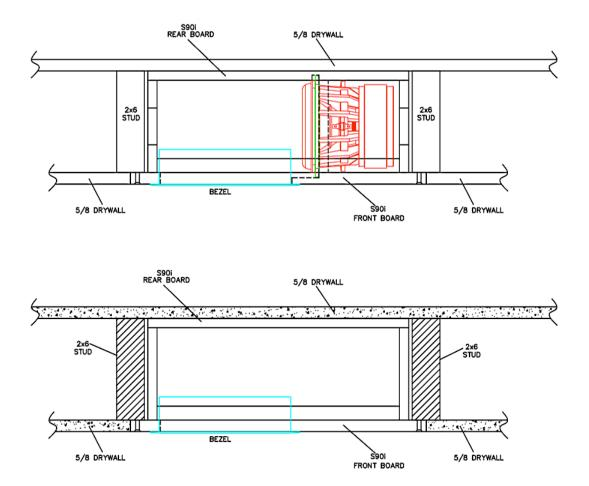
The front board of the S90 is made from <sup>5</sup>/8" MDO plywood, which presents a smooth, paintable finish surface similar to dry wall. It can be butted up against the <sup>5</sup>/8" dry wall, taped, and spackled, and painted like any other section of wall. It will also readily accept skim-coating if the construction calls for plaster walls.
