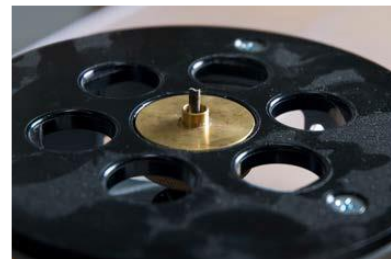
(Bottom of the Router with bushing and bit installed)
