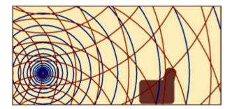
By contrast, the Sage L75 speakers radiate sound as a "line source". The sound moves into the room as an expanding cylinder, rather than as an expanding sphere — as though from a vertical line suspended in space.
