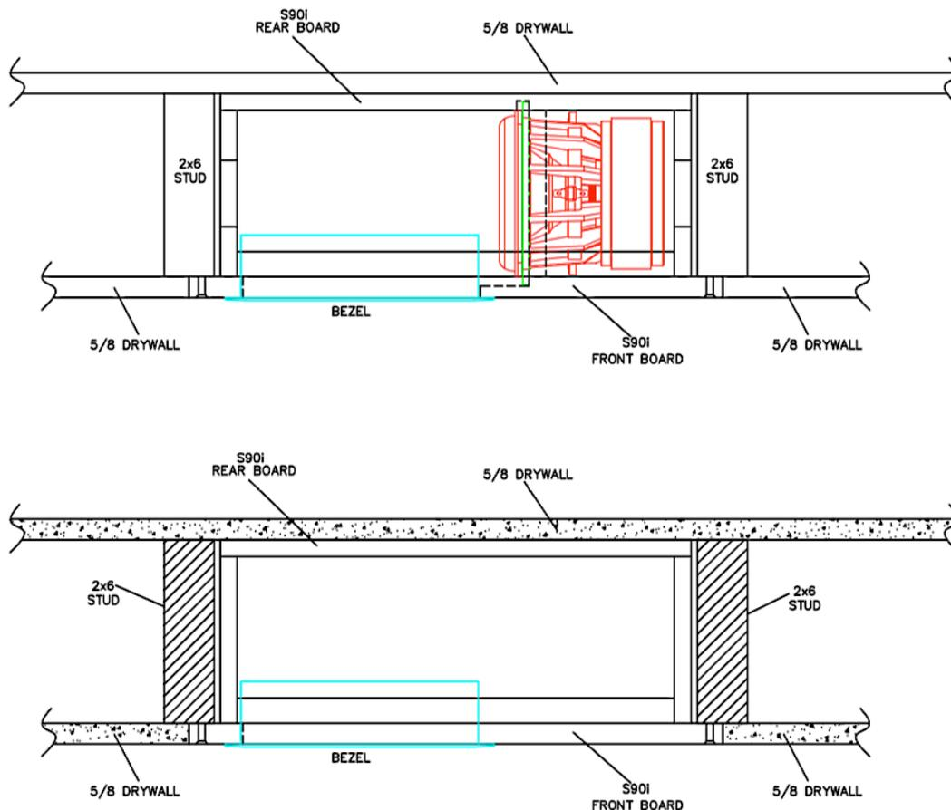
The front board of the S90i is made from  $\frac{5}{8}$ " MDO plywood, which presents a smooth, paintable finish surface similar to dry wall. It can be butted up against the  $\frac{5}{8}$ " dry wall, taped, and spackled, and painted like any other section of wall. It will also readily accept skim-coating if the construction calls for plaster walls.
