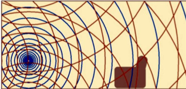
By contrast, the Sage L75i speakers radiate sound as a “line source”. The sound moves into the room as an expanding cylinder, rather than as an expanding sphere — as though from a vertical line suspended in space.
