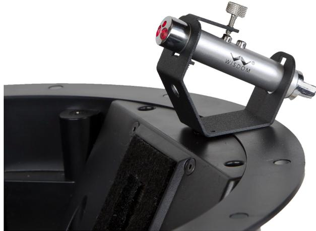
**8. If the IC-LAT Laser is used:** Turn the laser on the IC-LAT on by rotating the thumbscrew slowly in a counter-clockwise direction until the laser is activated. Rotate the speaker module until the IC-LAT laser is pointing to the desired listening position. Tighten the four screws that control the dog-ears until the speaker module is fixed tightly to the ceiling.
