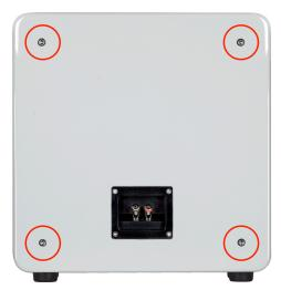
3. Use a metric #5 Hex key/Allen wrench to remove the four x 30mm screws that mount the rubber feet to the bottom of the subwoofer.
