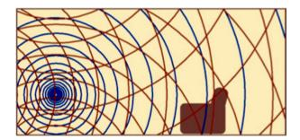
By contrast, the Wisdom Series LS3 speakers radiate sound as a "line source". The sound moves into the room as an expanding cylinder, rather than as an expanding sphere — as though from a vertical line suspended in space.
