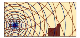
By contrast, the Wisdom Series LS4 speakers radiate sound as a "line source". The sound moves into the room as an expanding cylinder, rather than as an expanding sphere — as though from a vertical line suspended in space.
