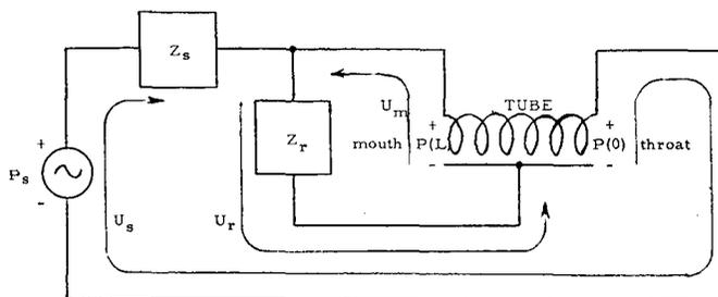
FIG. 4. Equivalent acoustical circuit of the Transflex.
