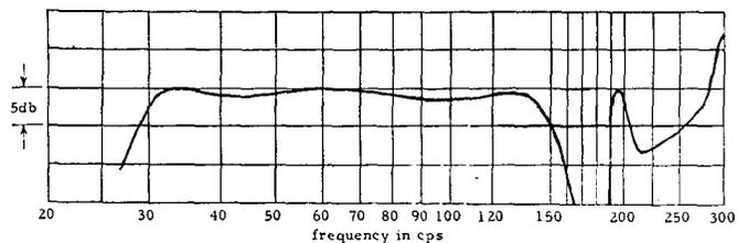
FIG. 8. Theoretical frequency response of the Transflex.
